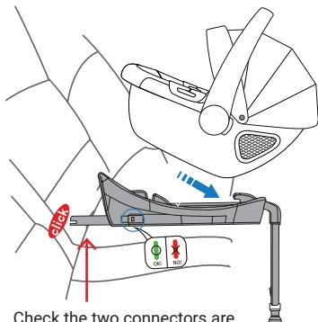
Check the two connectors are fastened correctly by trying to pull the base multiple times.
